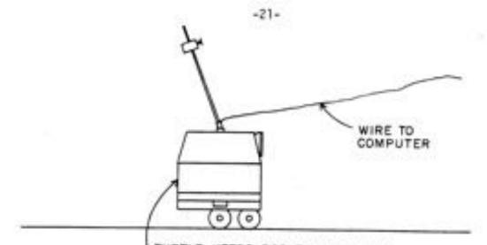
TURTLE KEEPS ROD FROM FALLING BY MOVING FORWARD AND BACK. POTENTIOMETER IN HINGE PROVIDES INFORMATION FOR FEEDBACK.
